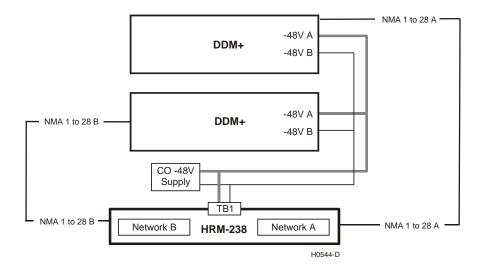
Figure 4. Recommended Network Setup for DDM+ Type Shelves
